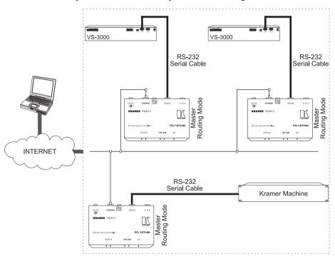
Figure 5: Connecting the FC-1ETHN in the Master Routing Mode
